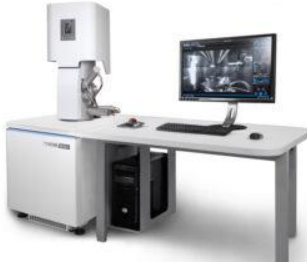
Figure 4. TESCAN's SEM equipment.
